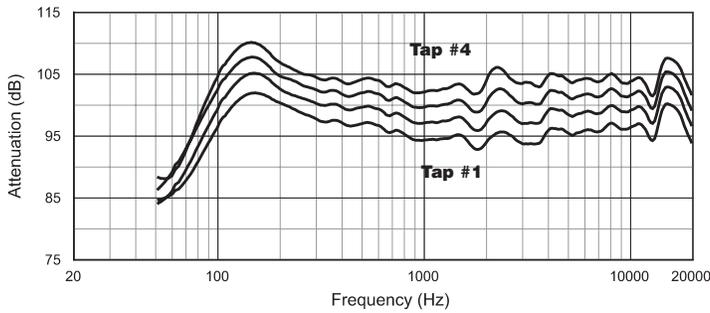
Frequency Response, in half-space with 70.7V input, taps #1 through #4. For 100V input, raise each curve 3 dB.
