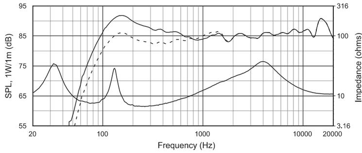
Frequency Response, on axis in half-space ( $2\pi$ , solid line) and full-space ( $4\pi$ , dotted line), in thru (8 ohm), with Input Impedance
