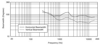
Measurements obtained in bi-amplified crossover mode
