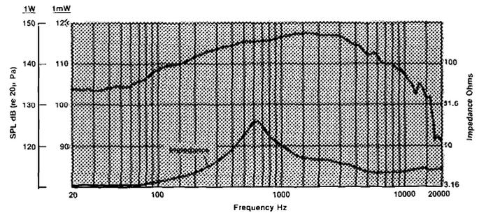
Frequency response and impedance modulus of Model 2426H coupled to a 25 mm (1 in) diameter terminated plane-wave tube. This is the power response of the transducer, and is the frequent response that will be obtained on a true full-bandwidth constant-directivity horn design, such as JBL's 2360 series of Constant Coverage Bi-Radial Horns.
