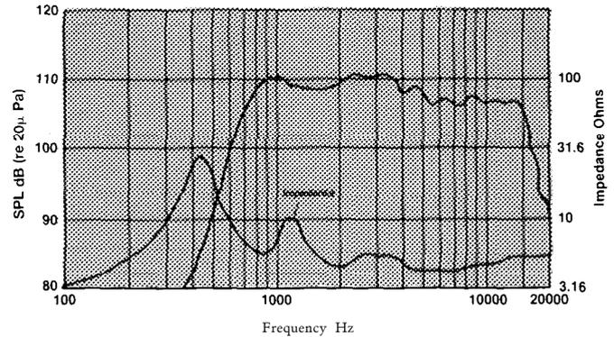
Frequency response of the 2426H coupled to a JBL 2370 Flat-Front Bi-Radial horn, measured on-axis at a distance of 1 meter with a 1 watt (2.83 V RMS) input in a reflection-free environment, with impedance vs. frequency curve. The increased high-frequency output is due to the horn design's increasing directivity in the vertical plan.
