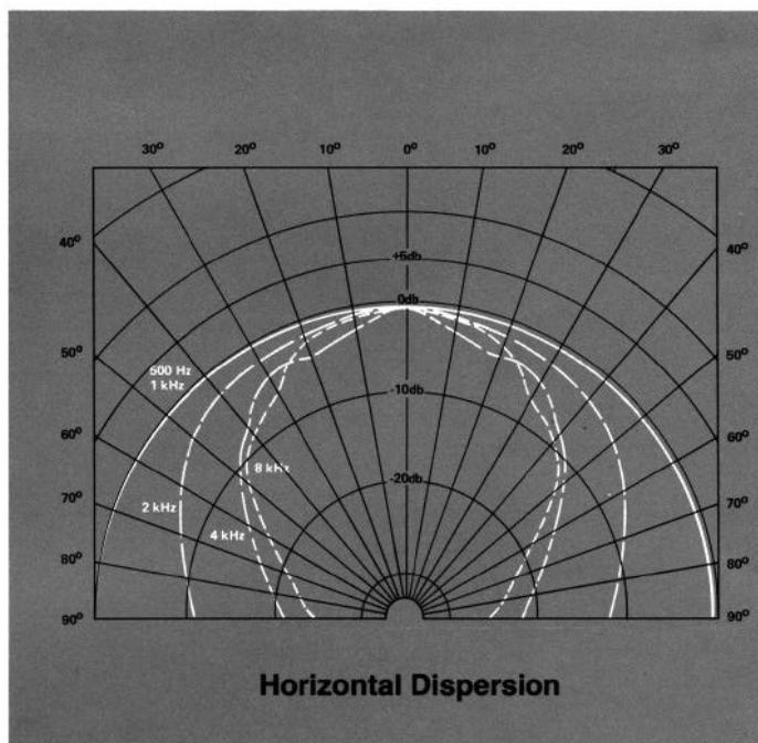
Above curves taken in hemispherical free-field conditions with the microphone at 7 m (24 ft) from the system. Power fed to the 4380 was adjusted to provide the same 0 dB reference for each curve.
